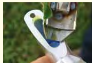
... and let several drops flow onto refractometer prism.
